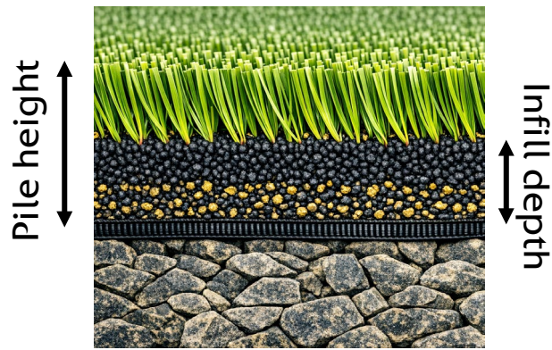
Filled: infill depth is at least 50% of pile height
